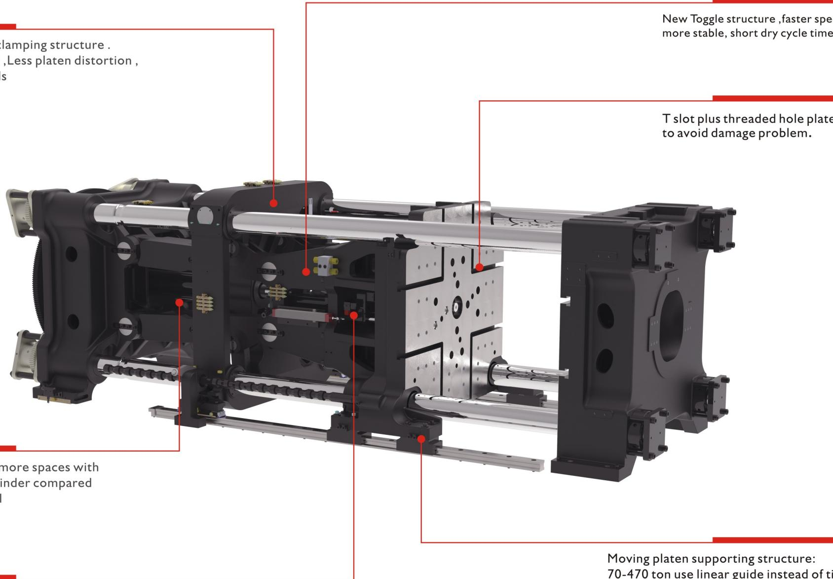
Patented pneumatic fast forced resetting connector, assemble & disassemble easily, adapted to all ejector structure.
