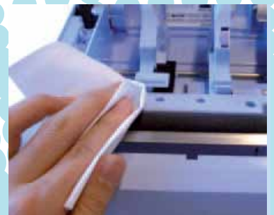
Cleaning rollers by presaturated Cleaning Cards
