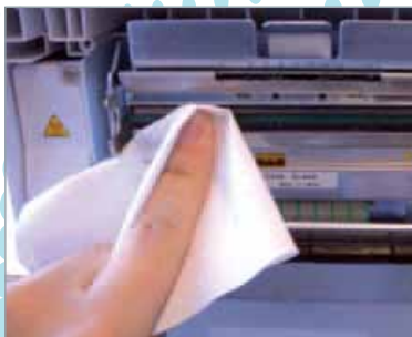
Cleaning print head by presaturated Cleaning Cards
